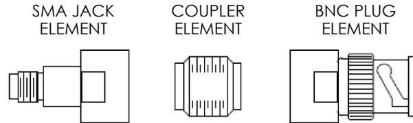
BAK400 CONSISTS OF 8 IDENTICAL COUPLER ELEMENTS AND 2 EACH OF THE FOLLOWING CONNECTOR ELEMENTS, A TOTAL OF 40 ELEMENTS.
